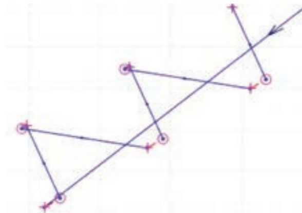
Figure 8: Section of the infill trajectory. Several discontinuous segments are shown.
